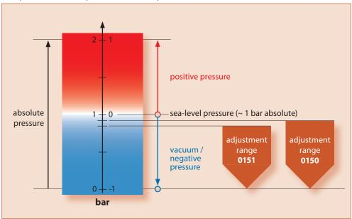
**Indication:** Desired switching points within the range of the vacuum have to be indicated relatively to the atmospheric pressure (normal pressure).
