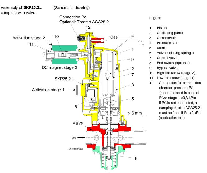
Setpoint adjustment «PGas» is made manually by turning the setting screws (10 and 11), which act on the setpoint spring.
