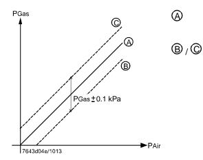
Gas / air ratio for stoichiometric combustion
