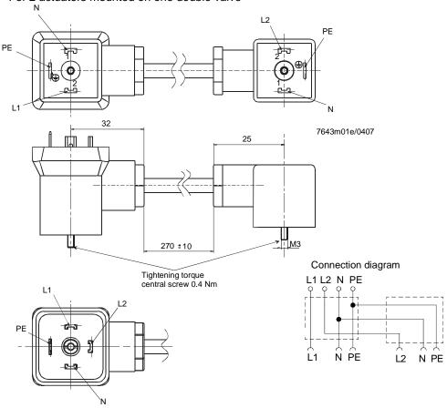
Adapter plug AGA62.2... (only SKP25.2...) - For 2 actuators mounted on one double valve
