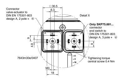
Adapter plug AGA62.000A000 - For 2 actuators mounted on one double valve
