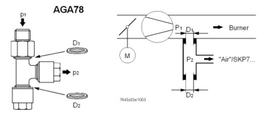
The reducing T-piece AGA78 is supplied ready for mounting, with D1 = 1.5 mm and D2 = 1.7 mm.
