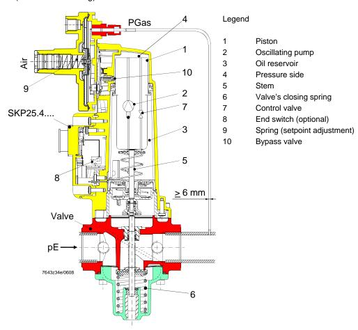
Setpoint adjustment «PGas» is made manually by turning the setting screw, which acts on the setpoint spring (for setpoint springs, also refer to «Accessories»).
