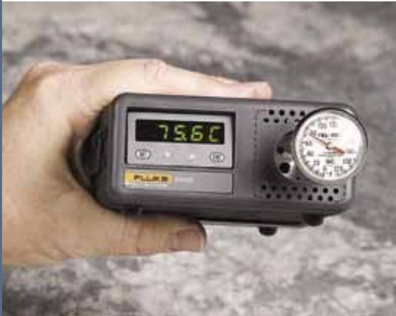
Temperature sensor calibration is easy with a handheld dry-well.
