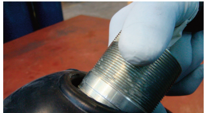
- Remove the gas valve, tilting slightly
