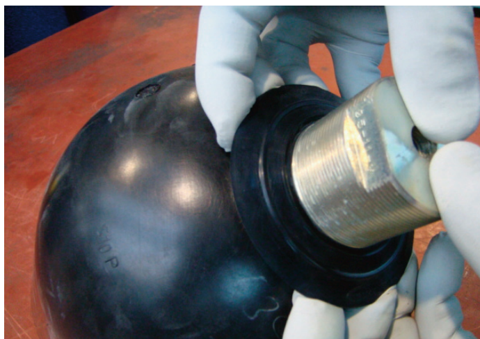
- Remove the gas valve, by pulling the bladder.
