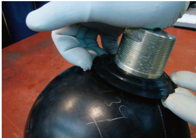
- Remove the gas valve, tilting slightly
