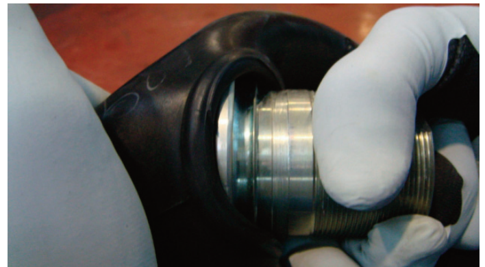
- Remove the gas valve, by pulling the bladder.
