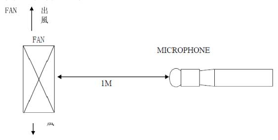
NOISE IS MEASURED AT RATE SPEED IN ACOUSTIC CHAMBER WITH B&K SOUND LEVEL METER. BACKGROUND NOISE:MAX 18dB(A).
