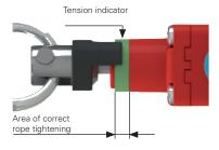
All switches are provided with a green ring that shows the area of the correct tightening of the rope. The installer has only to tighten the rope until the black indicator will be in the middle of the green area. With this setting, the switch can be reset by pulling the blue knob to close the electrical safety contacts.
