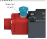
If the tension indicator is in the green area, the electrical safety contacts can be closed by pulling the blue knob. The reset status can be identified quickly by the green ring under the blue knob.
