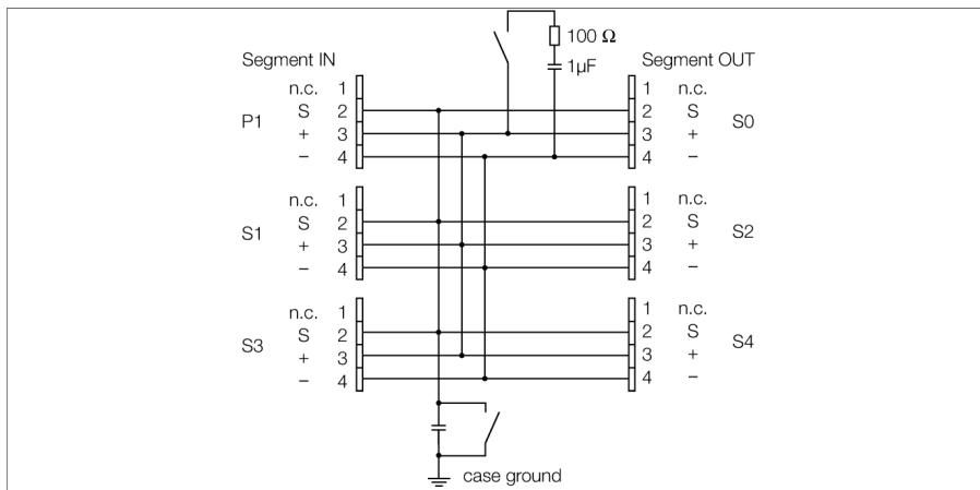
The 4-channel Ex junction box JBBS-49-E413/EX is designed for FOUNDATION™ fieldbus systems.
