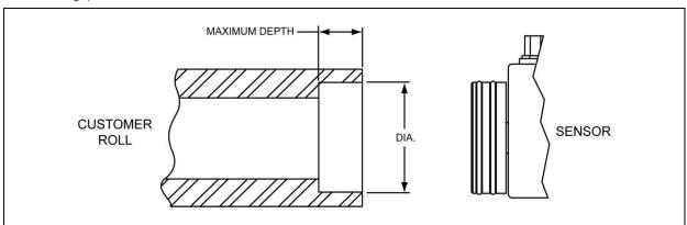
52.0 +.05/-.00 mm diameter; 0.53 in. (13.5 mm) maximum depth for 5 lb, 50 lb, 2 kg, and 25 kg sensors 62.0 +.05/-.00 mm diameter; 0.76 in. (13.9 mm) maximum depth for 150, 330 and 500 lb, 75 kg, 150 and 250 kg sensors
