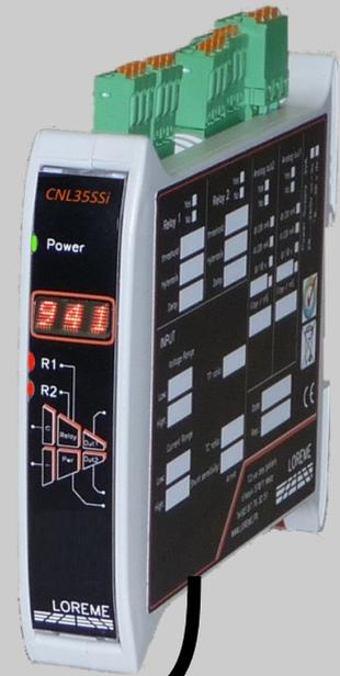
The CNL35SSi converts a SSi information provided by a single-turn or multi-turn positional encoder into one or two analog outputs and with up to 2 alarms relays.
