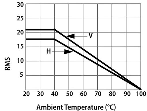
**V:** Heatsink mounted to a **vertical** surface
