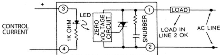
Control Current varies with control voltage. For details, see "Control Current Calculation" on page 17.
