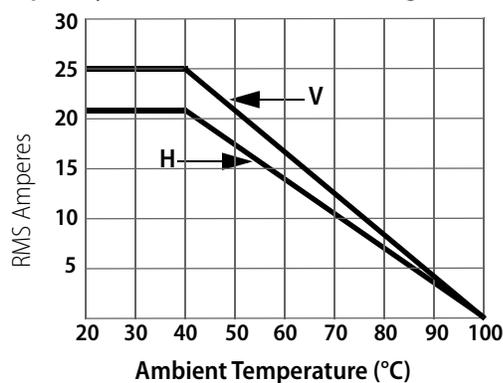
**V:** Heatsink mounted to a **vertical** surface
