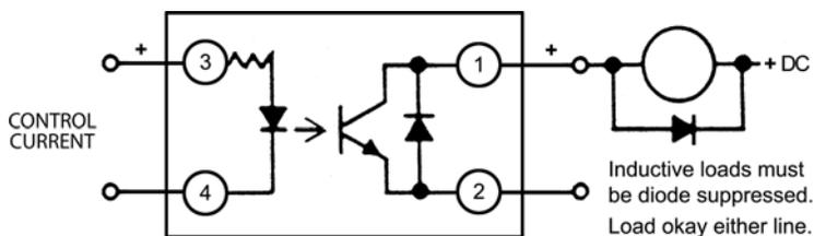
Control Current varies with control voltage. For details, see "Control Current Calculation" on page 17.
