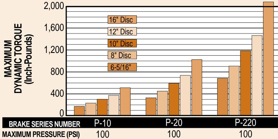
These graphs have been included for quick reference. Intended for use as a general guide, they reflect the maximum torque values possible with each brake and disc combination.
