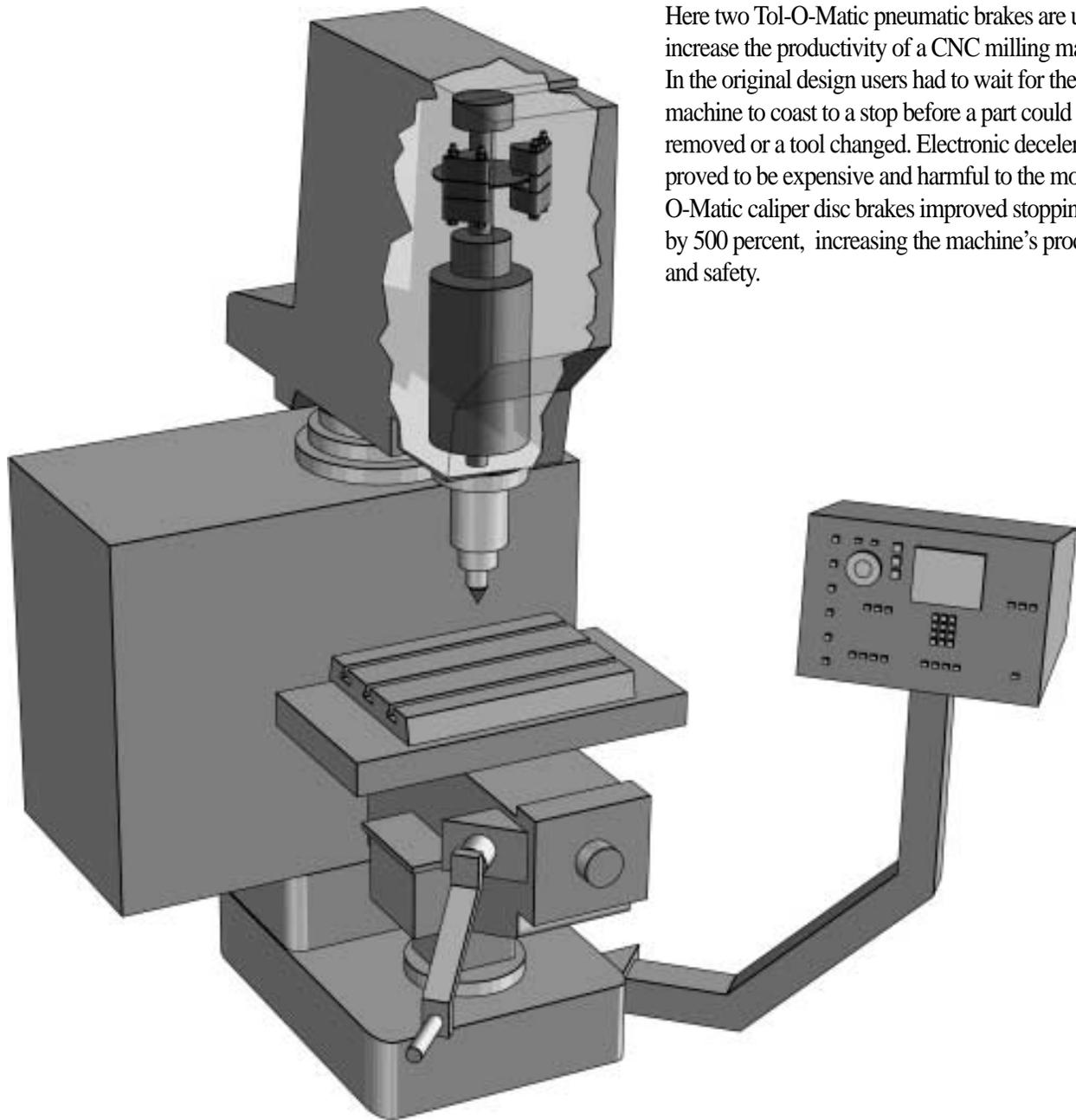
Here two Tol-O-Matic pneumatic brakes are used to increase the productivity of a CNC milling machine. In the original design users had to wait for the machine to coast to a stop before a part could be removed or a tool changed. Electronic deceleration proved to be expensive and harmful to the motor. Tol-O-Matic caliper disc brakes improved stopping time by 500 percent, increasing the machine's productivity and safety.
