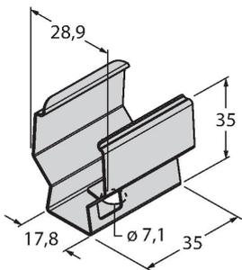
Snap bracket for mounting WLS28 work lights
