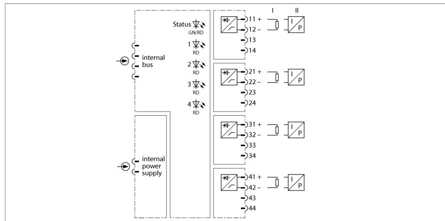
The output module AO401Ex is used for the connection of intrinsically safe analog actuators such as control valves or process indicators.
